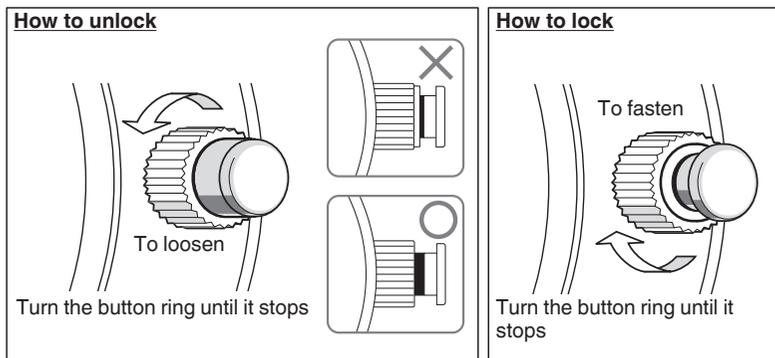
Turn the button ring counterclockwise (6 o'clock direction) to lower the slide cover gradually. Turn the button ring further until you can clearly see the guide line and the button ring can no longer be turned. Now the screw-lock type button is unlocked and can be operated.
