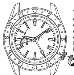
Turning the crown clockwise (12 o'clock direction): The hour hand is set back one hour.
