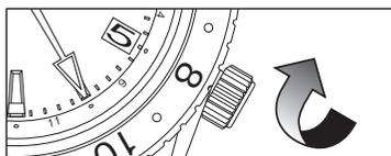
Turning the crown clockwise (12 o'clock direction):
